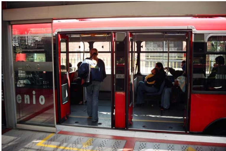
One of two sets of two 1.1 m-wide doors allowing rapid boarding and alighting on Bogotá’s BRT
