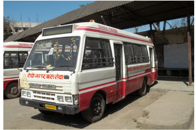
The buses procured under JNNURM are Swaraj Mazda minibuses with a seating capacity of 29 passengers. All buses are equipped with LED boards to display route information inside and outside the bus.
