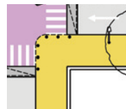
Figure 4.6 The boundaries of pedestrian spaces are defined by bollards to prevent encroachment by vehicles.
