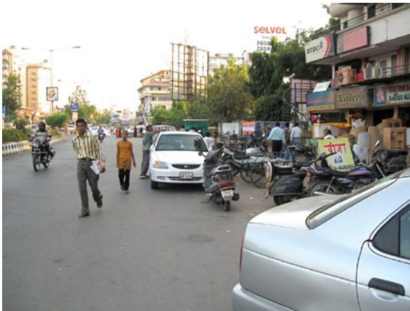
✗ Figure 2.40 When pedestrians encounter haphazardly parked vehicles, they generally walk next to moving vehicles because this part of the street offers the most direct route.
