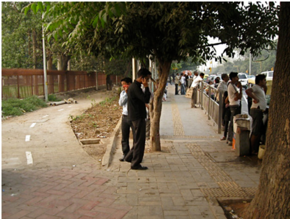
Figure 5.30 The cycle track is routed behind the bus stop to avoid conflicts between cyclists and waiting bus passengers.
