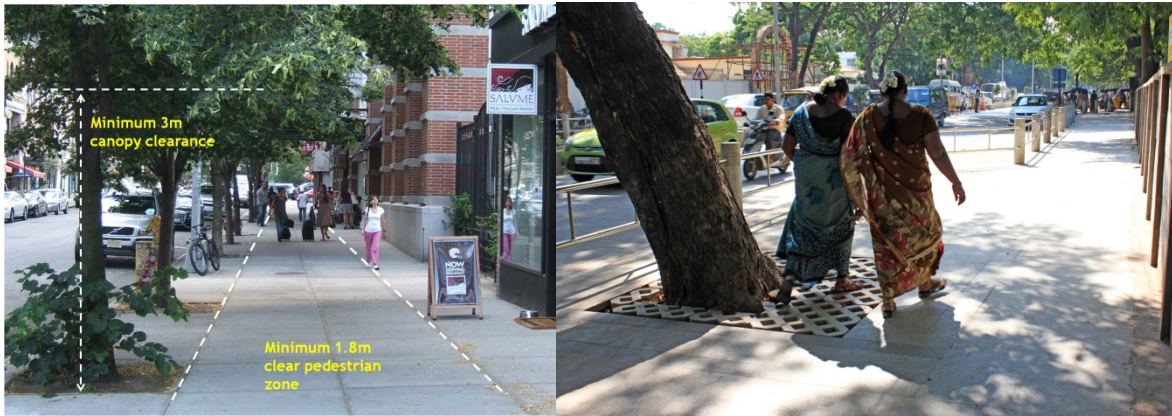
Figure 5. Placement of trees shall allow for a clear walking and cycling path. A 3m canopy height ensures better visibility for pedestrians (left). Tree will be protected with tree pits that allow unobstructed pedestrian movement (right).
