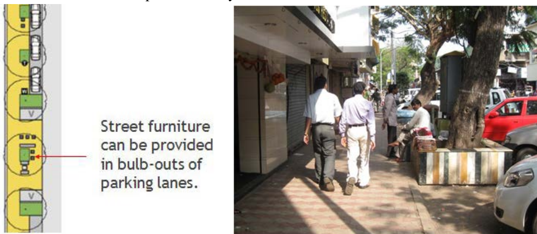
Figure 8. Street furniture shall be located where it does not obstruct pedestrian movement, such as in parking bulb-outs (left) or in the furniture zone (right)
