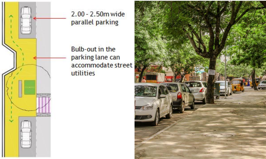
Figure 9. Parallel parking for cars is the most efficient parking layout, as compared to perpendicular and angular parking.
