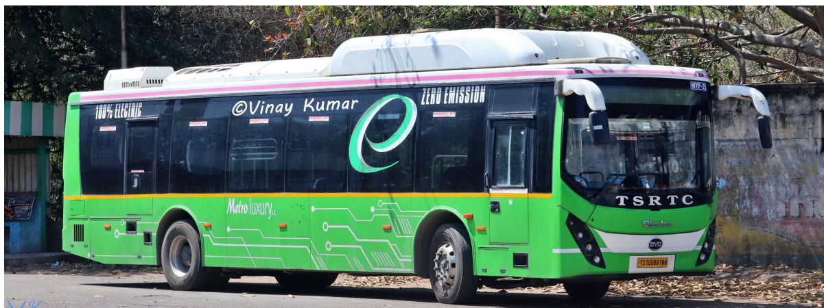
Figure 12 : TSRTC's 12m electric bus operated on Airport route in Hyderabad (Mofussil) 24
