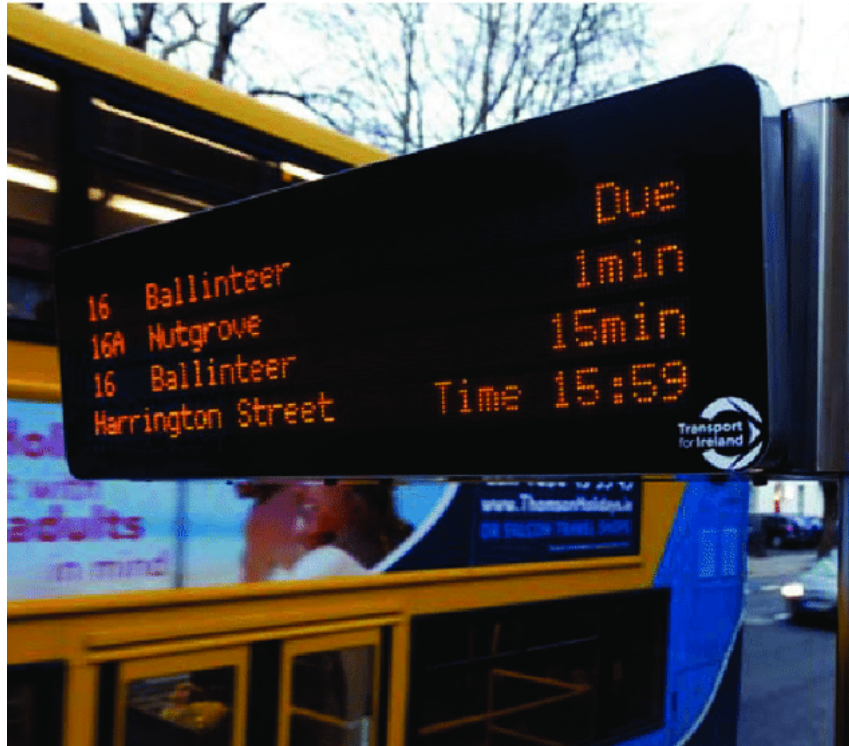
Dublin's bus stop features a digital display with the estimated time of arrival (ETA) Image source: Smart Dublin
