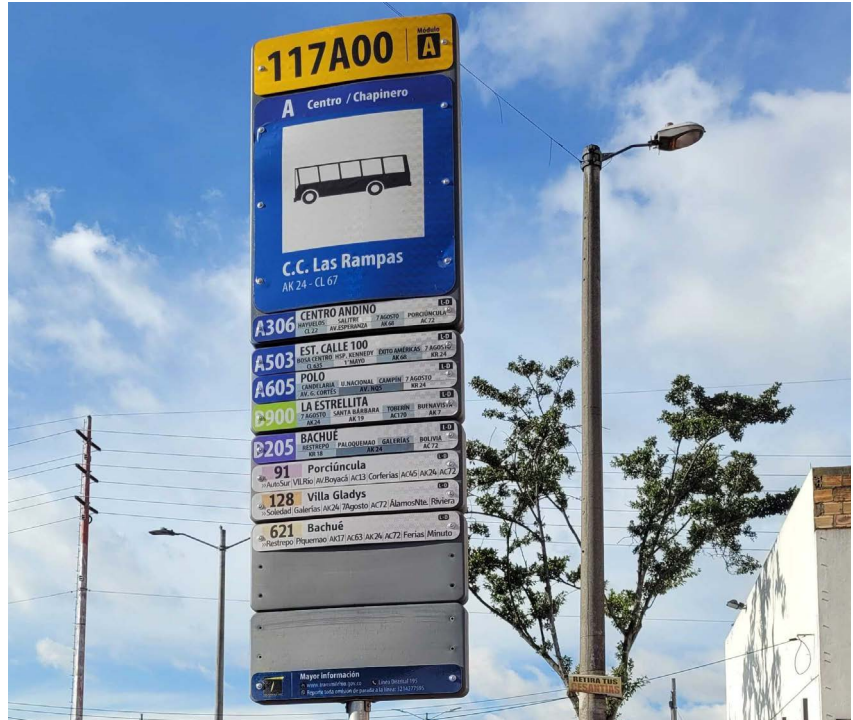
Bogotá’s bus stop pole signage has panels of bus route information that can be replaced in case of any changes Image source: ITDP India
