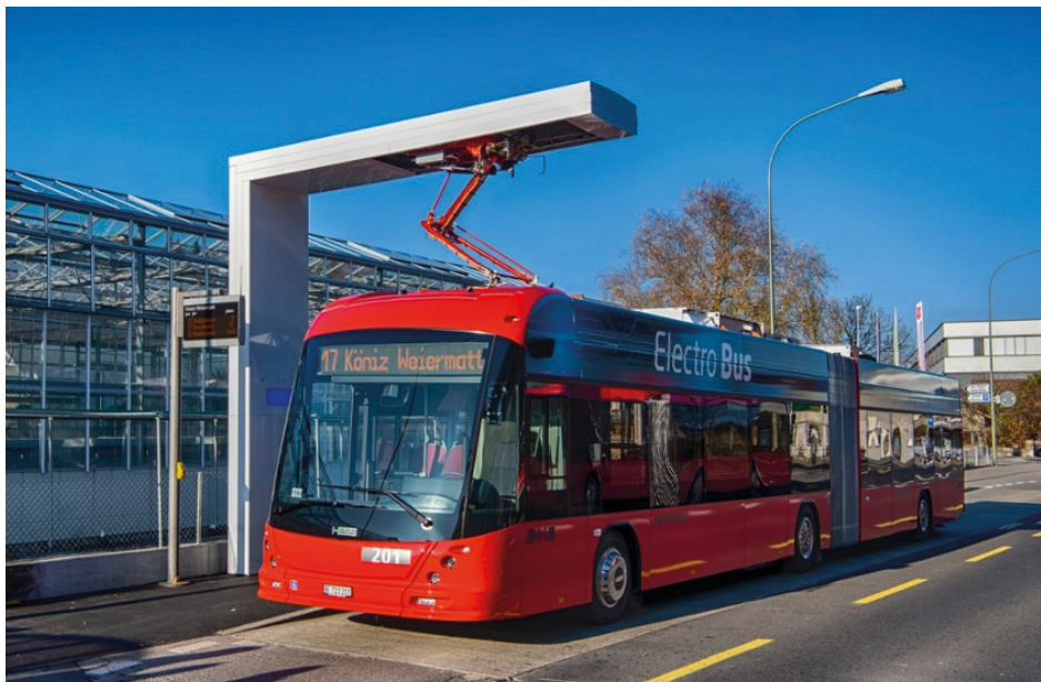
Figure 8: A hess bus using a roof-mounted Pantograph in Bern 21
