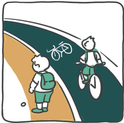
Segregated footpaths and cycle track
